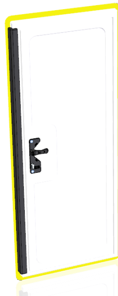
Figure 4: Bonding Surface Area
